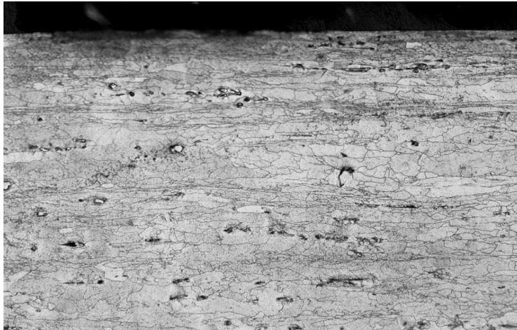
Figure 7 - Hot rolled Pb-(0.07%)Ca-(0.35%)Ag anode sheet
