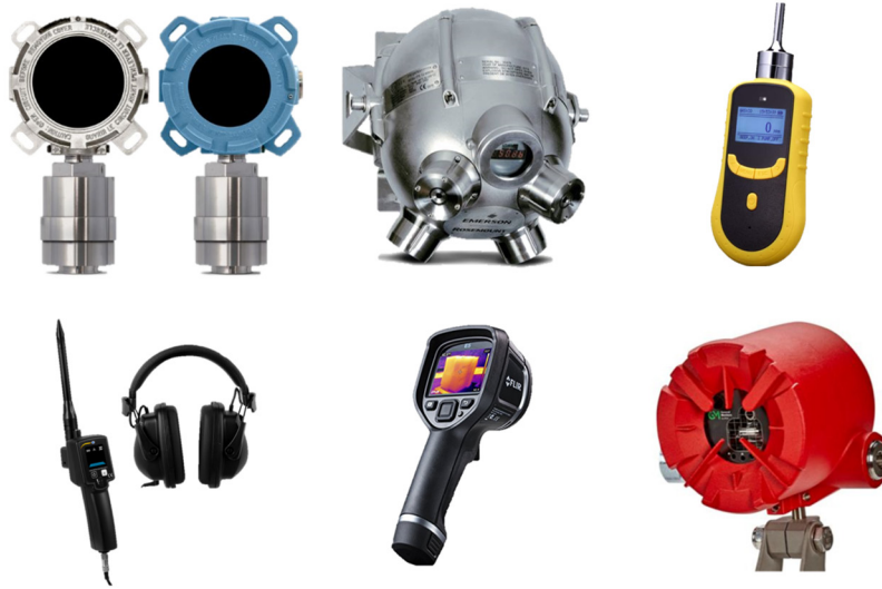
Figure 4: Common leak detectors used in hydrogen systems. Catalytic bead point sensor (top left [13]), ultrasonic area leak detector (top middle) [14], handheld electrochemical sensor with pump (top right) [15], handheld ultrasonic leak detector (bottom left) [16], handheld thermal imaging leak detector (bottom middle) [17], UV/IR flame camera (bottom right) [18]
